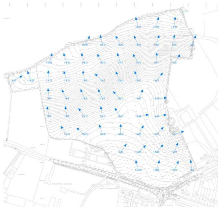
Figure 2 – Existing topography with approximate direction of fall
