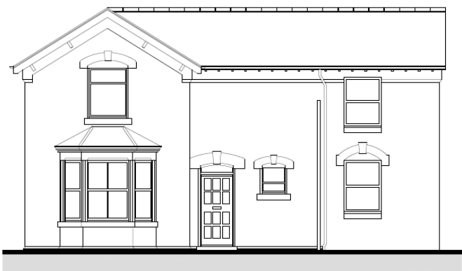
Existing Front Elevation
