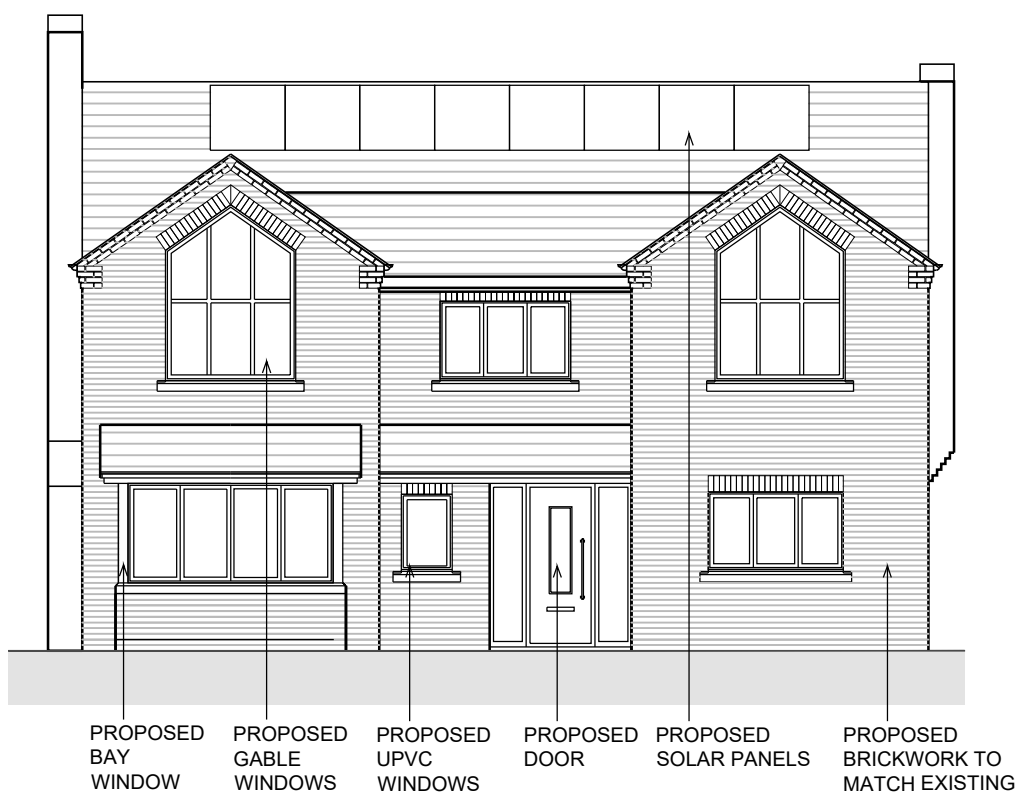
03 Front Elevation Scale 1:100
