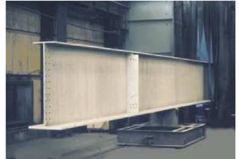
Steel beam emerging from an automatic blast cleaning unit
