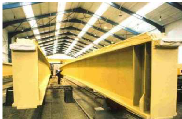
Airless spraying on steel bridge beams
