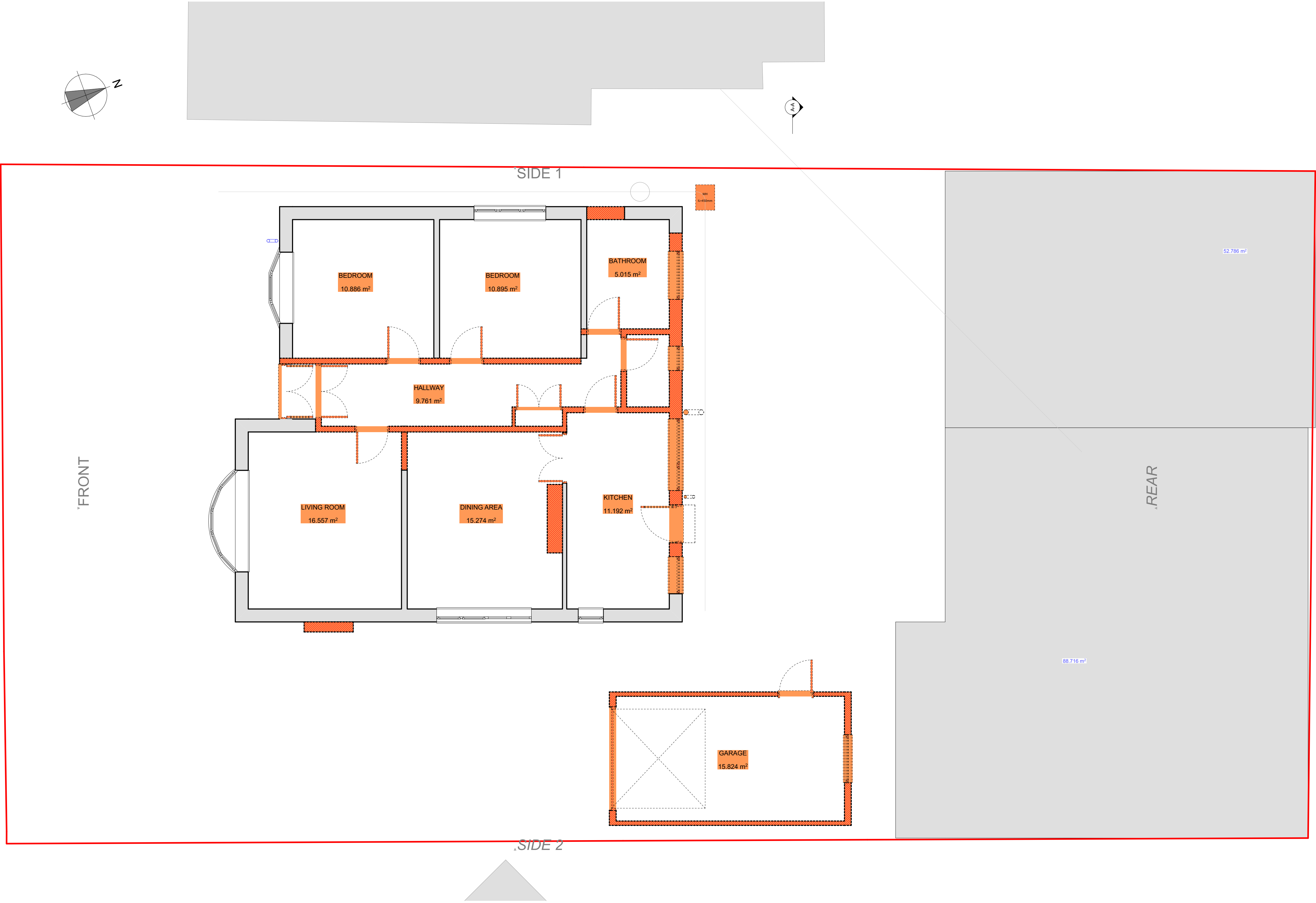
+00-Ground Floor Plan - Demolished
