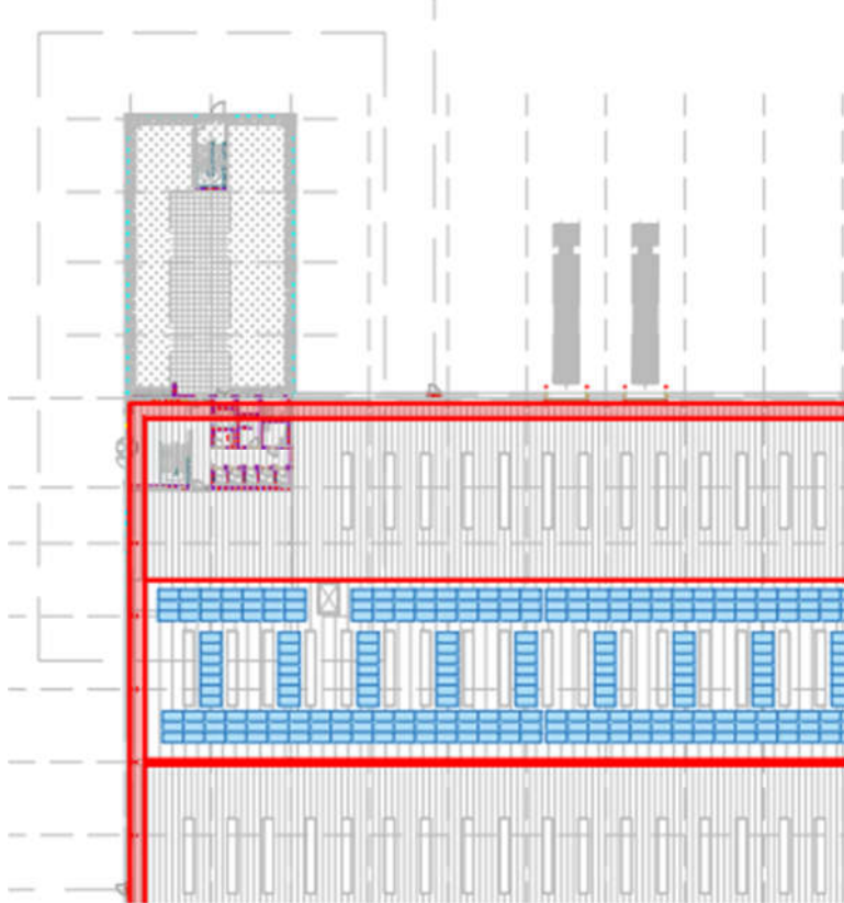
D. 003 – Roof access hatch locations for high level roof – Bardon 3
