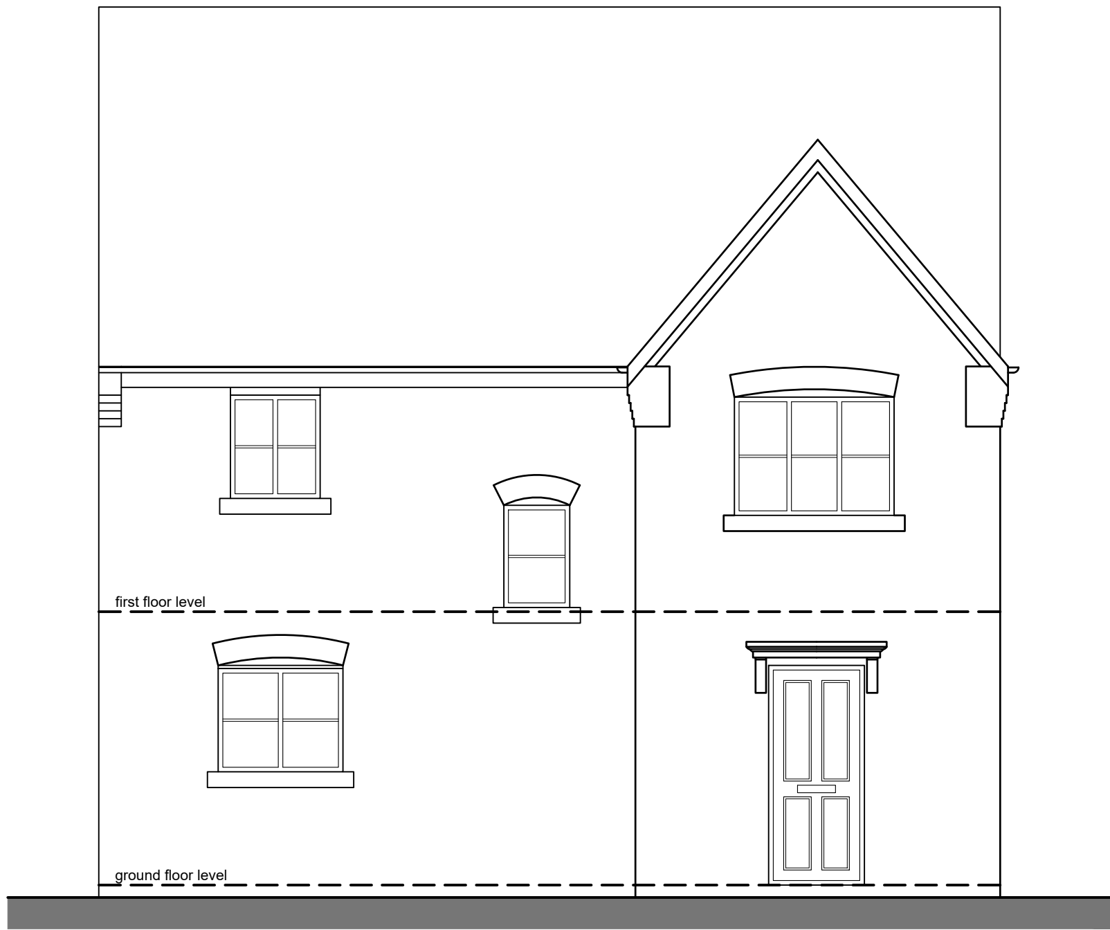
EXISTING FRONT ELEVATION (SOUTH) @ 1:50
