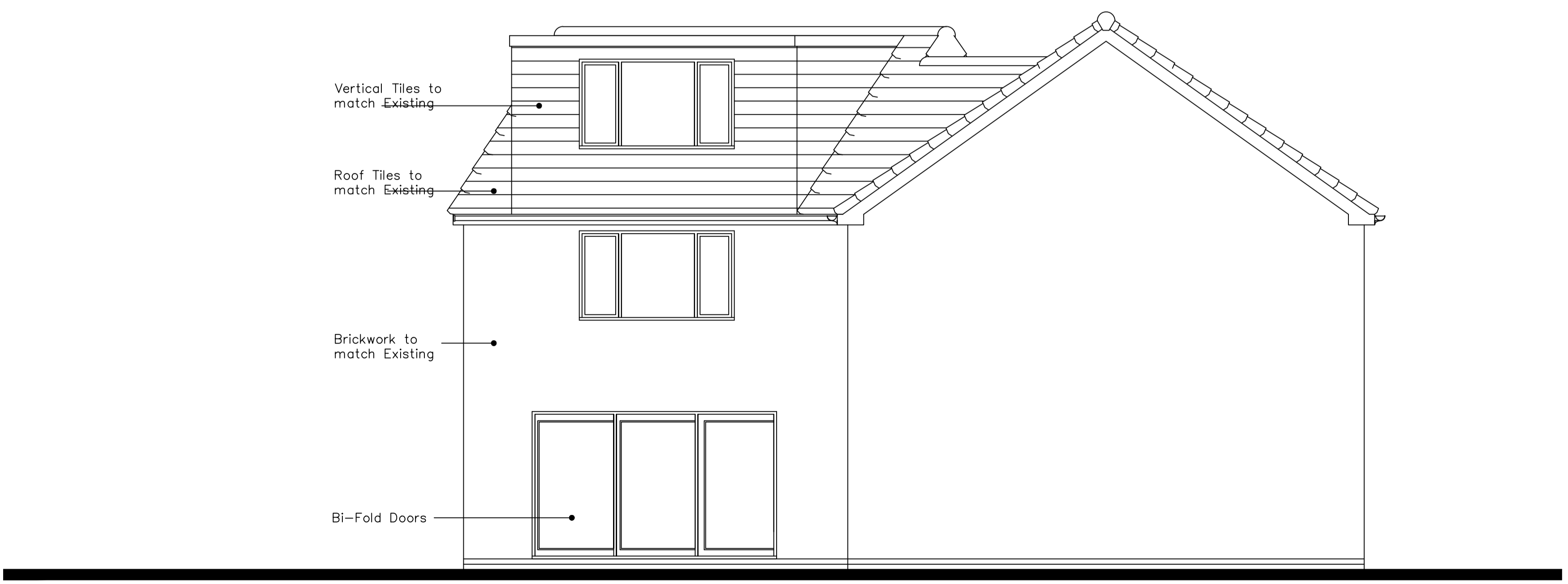
Proposed Gable Elevation Scale 1:50
