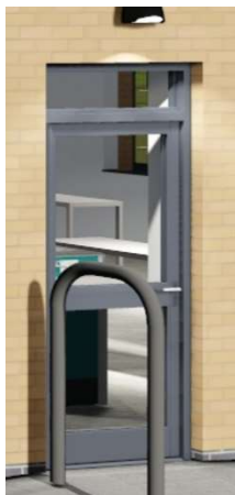
Figure 6: Single leaf door, aluminium frame with double-glazed infills
