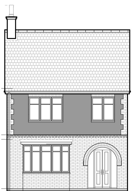
EXISTING FRONT ELEVATION 1:100
