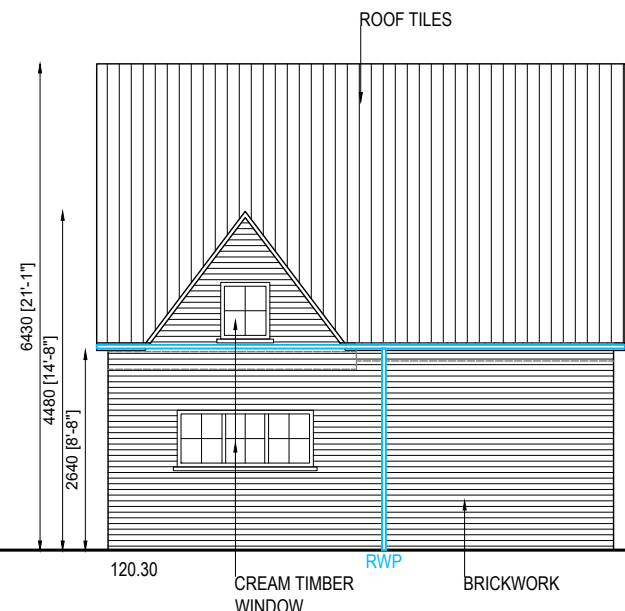
EXISTING GARAGE SIDE ELEVATION SCALE 1/100
