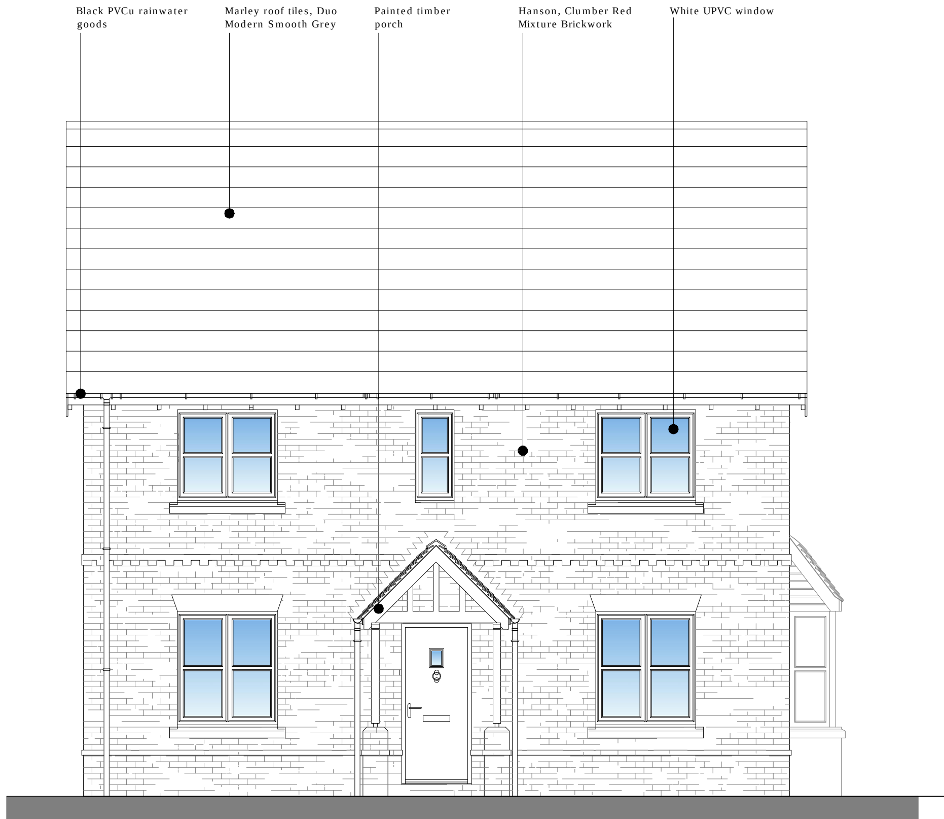
Front Elevation - As Existing
