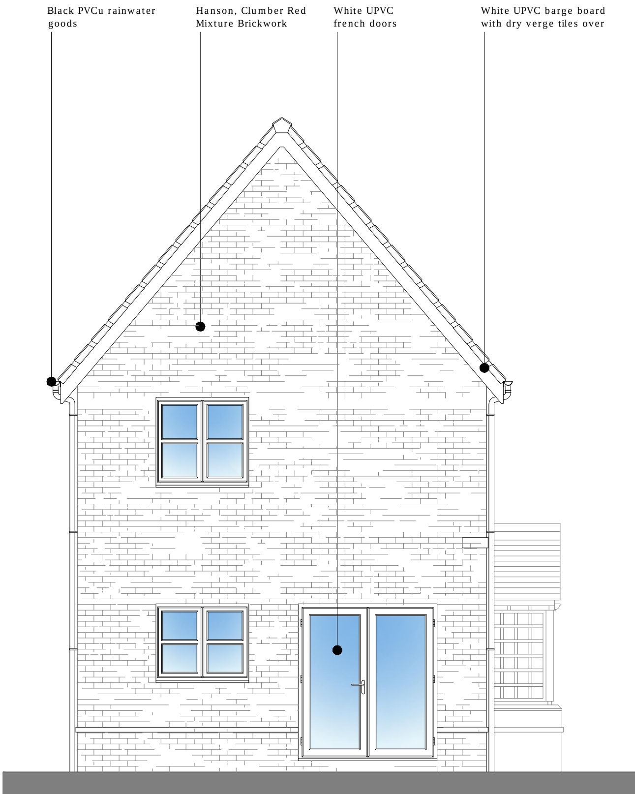
Side Elevation - As Existing
