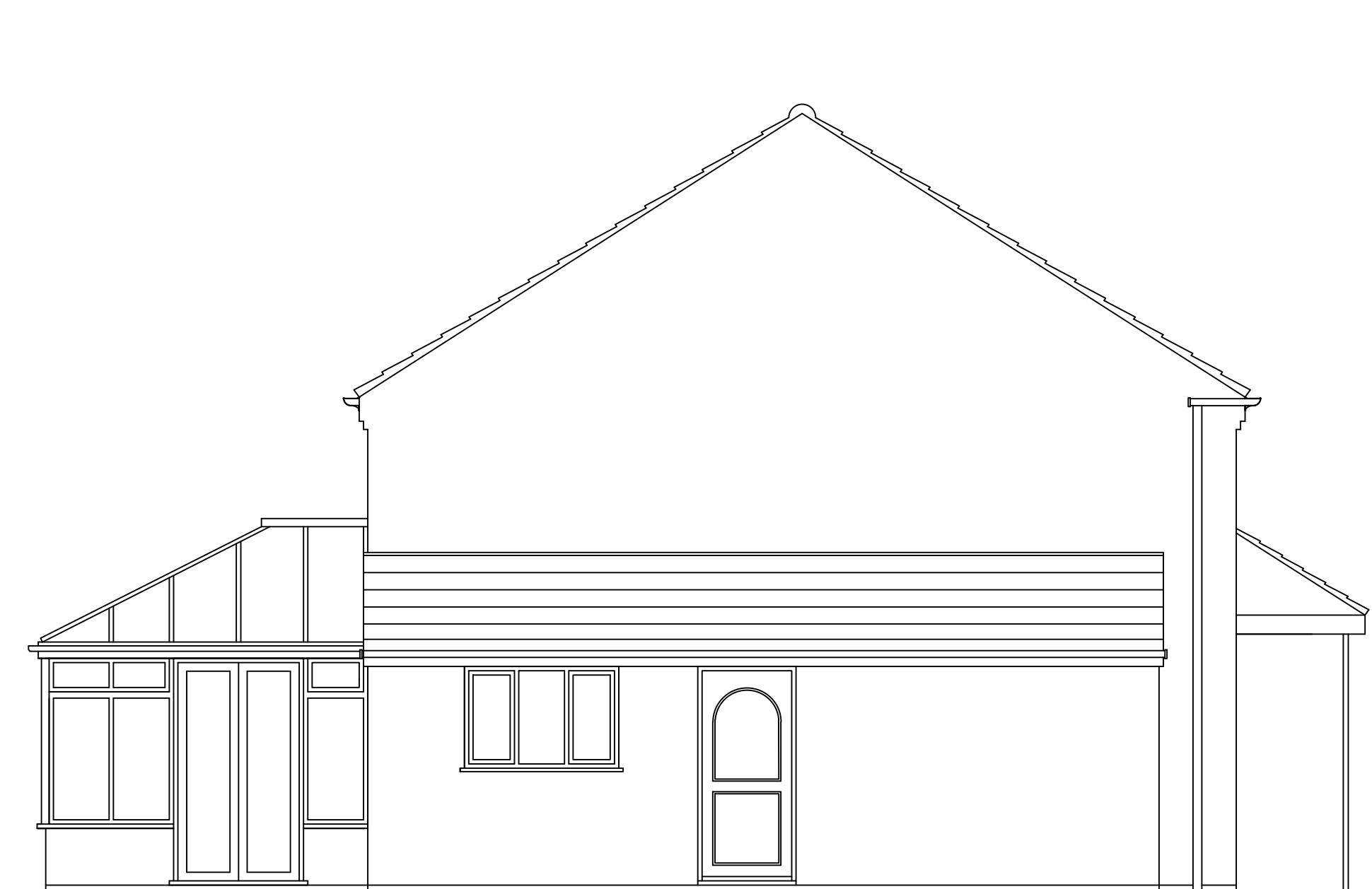
Existing Gable Elevation Scale 1:50
