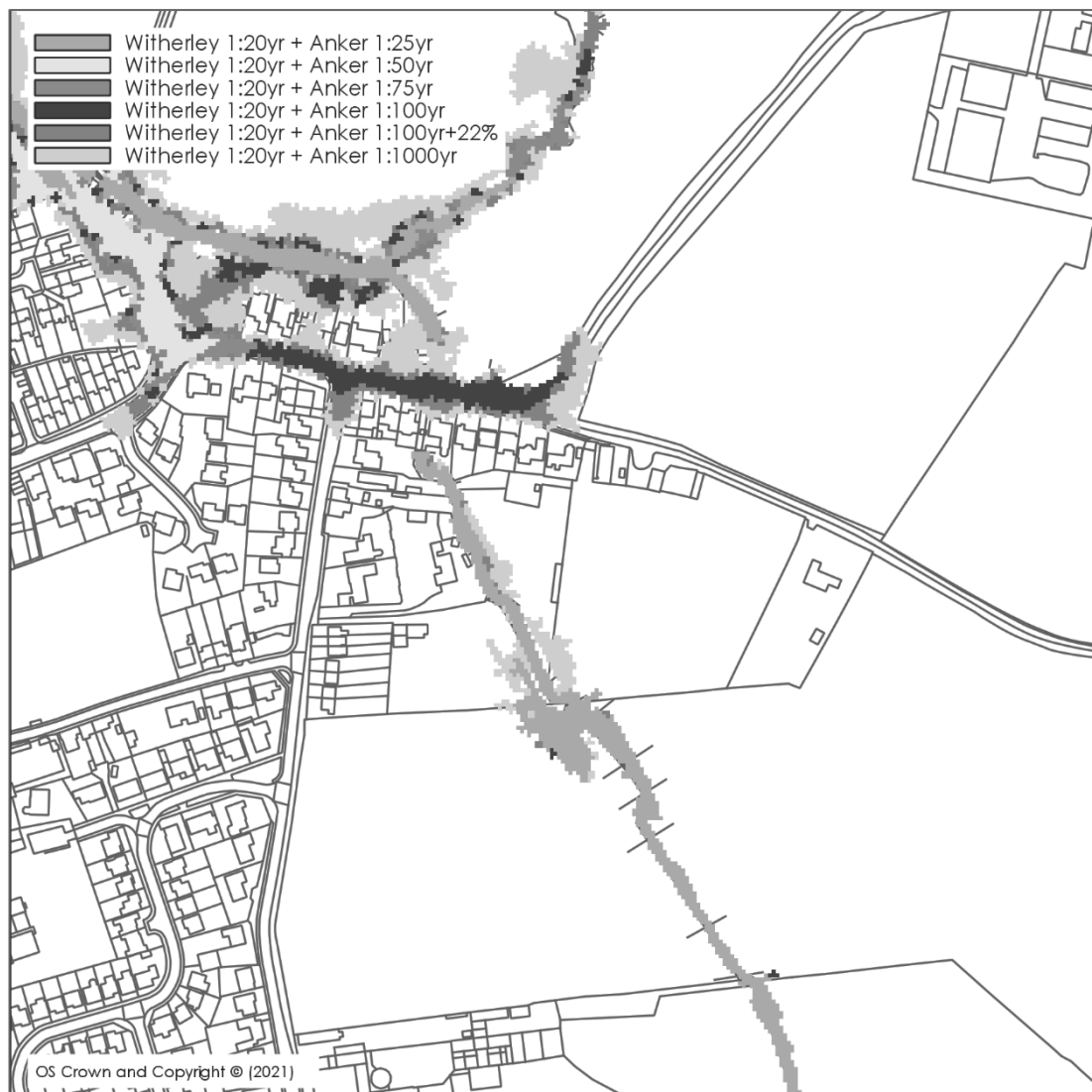
Figure 4-2: Floodplain extents: River Anker events
