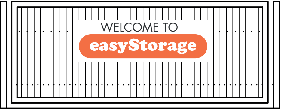
New electric sliding gate (2.2m high) with signage
