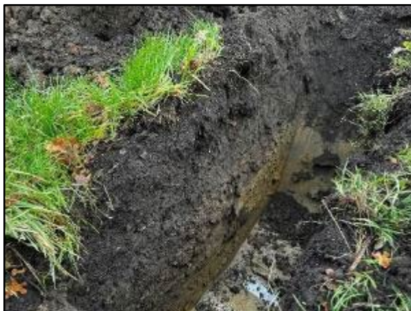
Photo 5 – A photo of TP03 where made ground was recovered.
