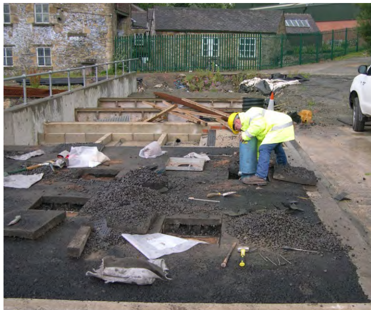
Figure 3 - In situ density tests post-trafficking.
