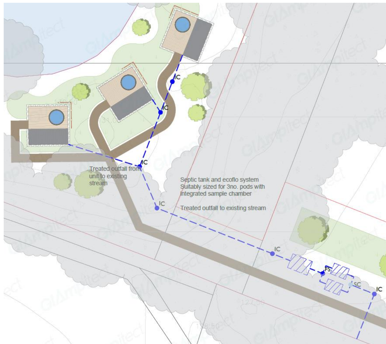
Figure 9. Proposed Drainage Plan
