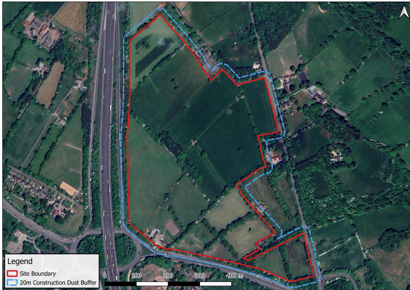
Figure 4: Construction Dust Buffers
