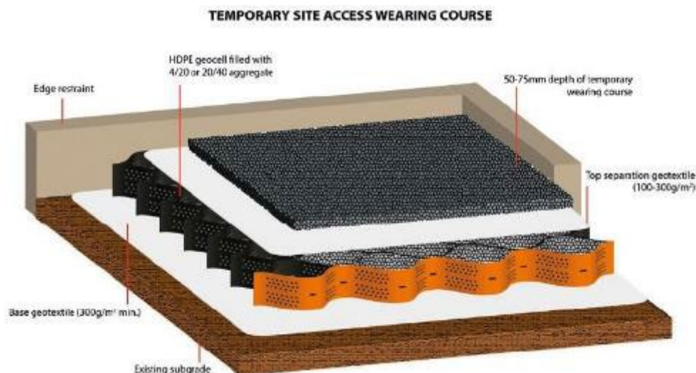
Image 2: Proprietary system – A geocell surface used during construction with a temporary hard wearing surface and a geotextile membrane to prevent mud from migrating down into infill (specifications and depths need to be confirmed by an engineer).
