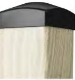
The post end caps are made of injection molded high quality nylon (PA6). PA6 has good wearing and impact strength and is UV stabilized. The end caps protect vertical placed posts to ensure long lifetime.
