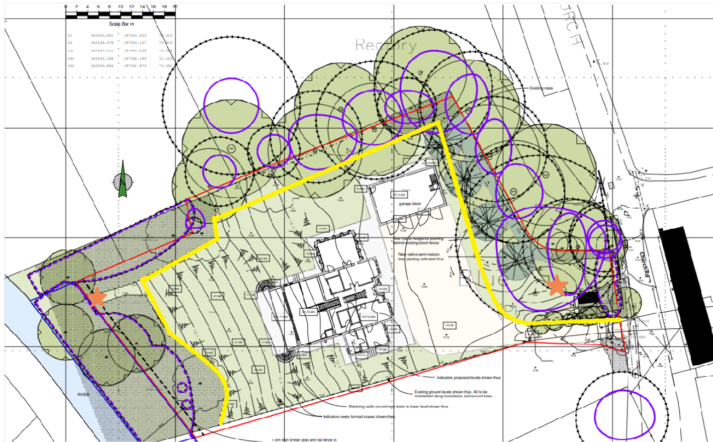
Figure 15 Revised Site Layout with new refugia (orange) and Heras fencing (yellow) locations (drawing extract: Hayward Architects, 2025. drawing no: 25 89 07H)
