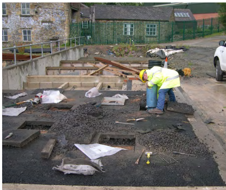
Figure 3 - In situ density tests post-trafficking.
