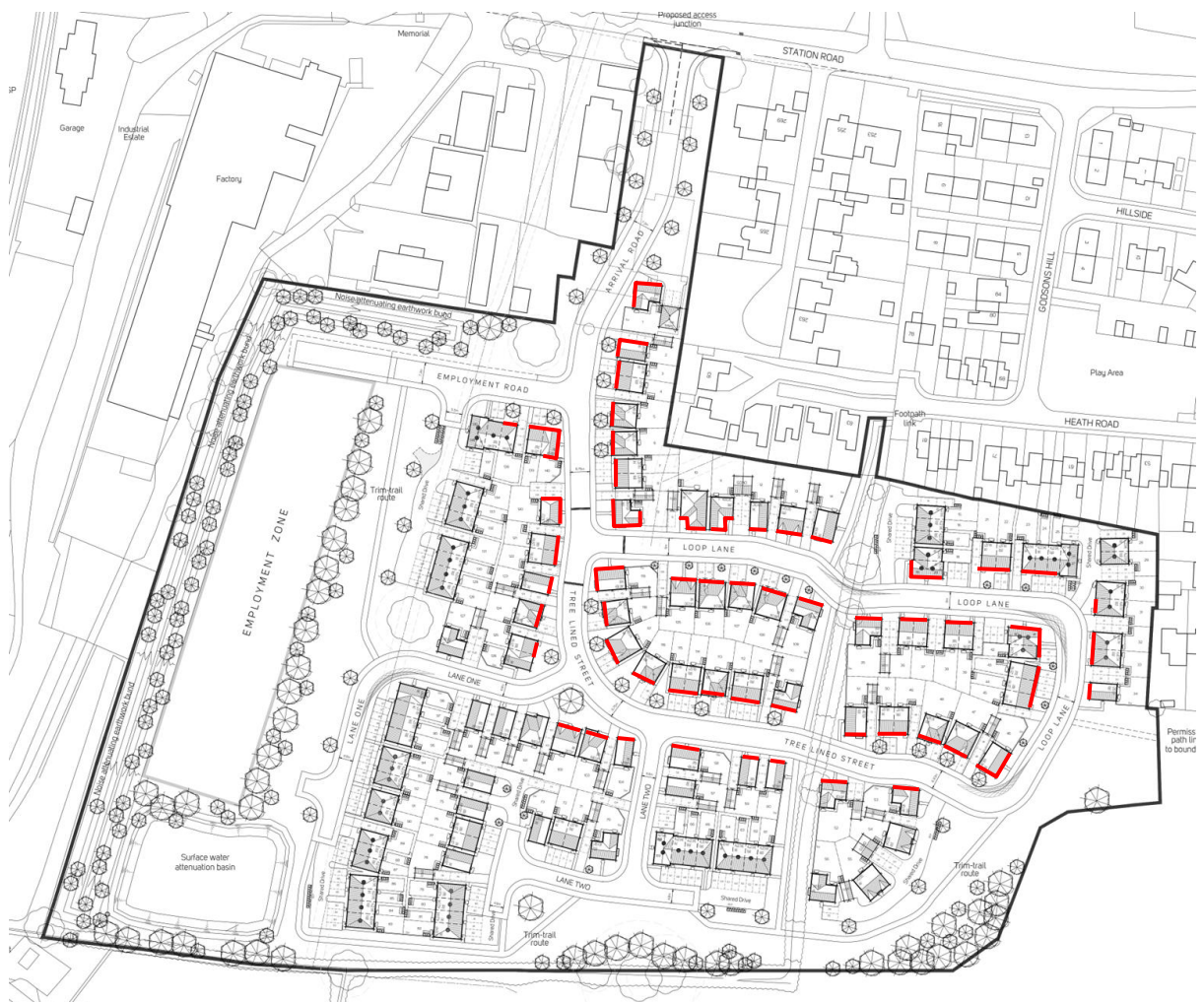
Figure 7. Bedrooms that will require dynamic thermal modelling to demonstrate compliance with Approved Document O
