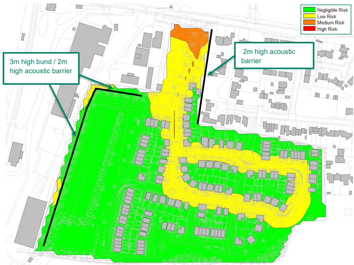
Figure 4. ProPG areas of risk, daytime, 1.5m above ground contour, L_{Aeq,16hour}
