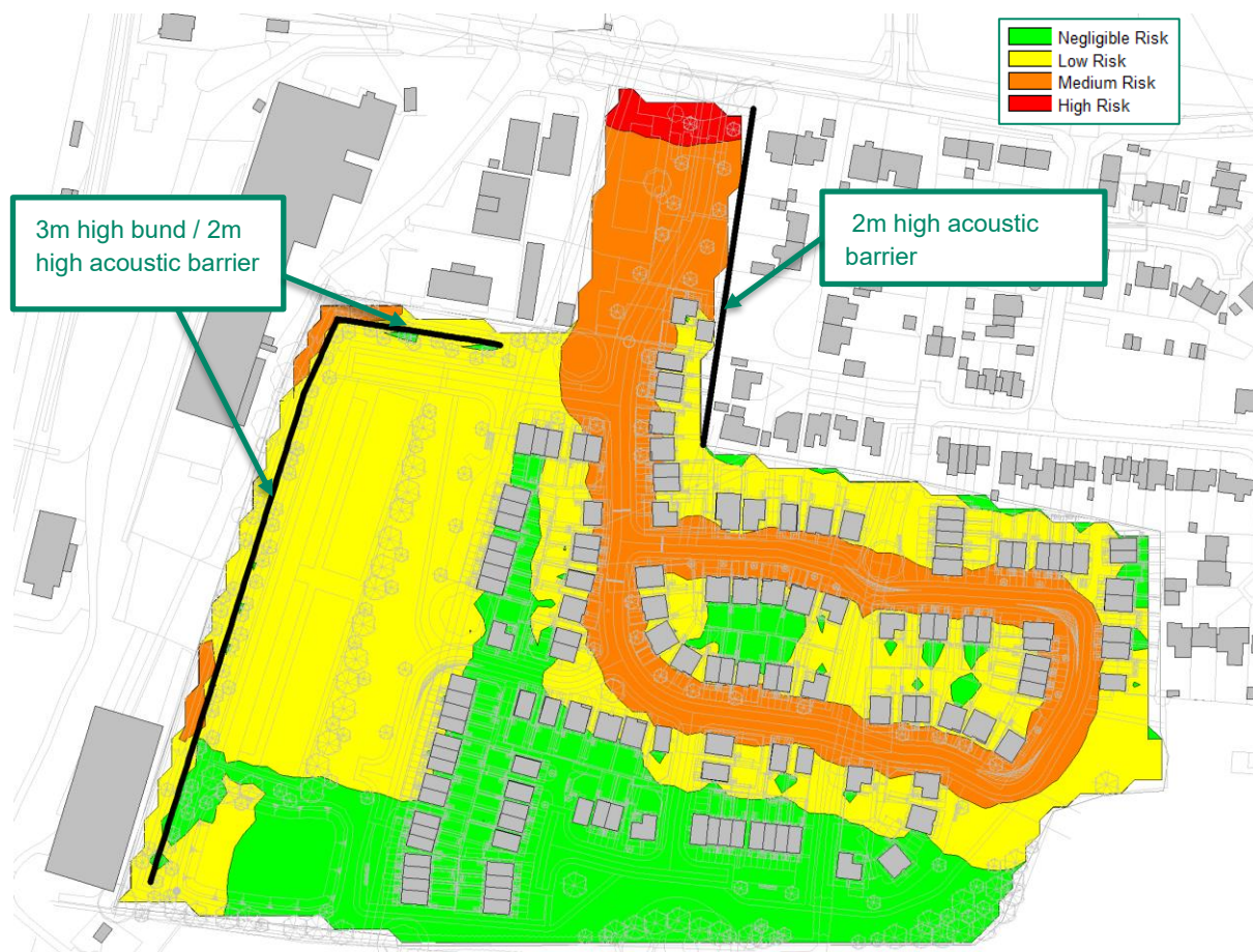
Figure 5. ProPG areas of risk, night-time, 4m above ground contour L_{Aeq,8hour}
