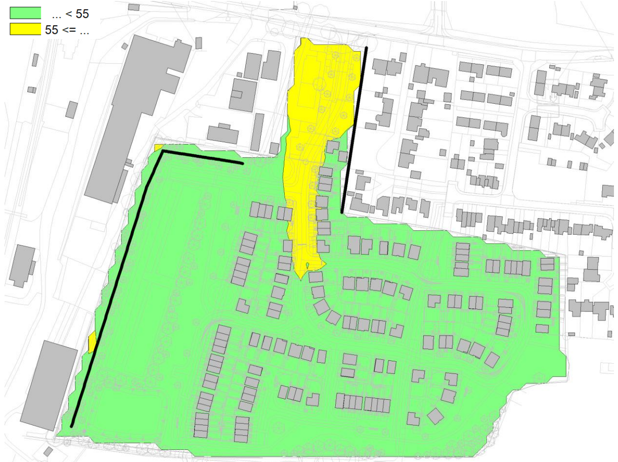
Figure 8. Noise contour daytime at 1.5m above ground, dB L_{Aeq,16\text{ hours}}
