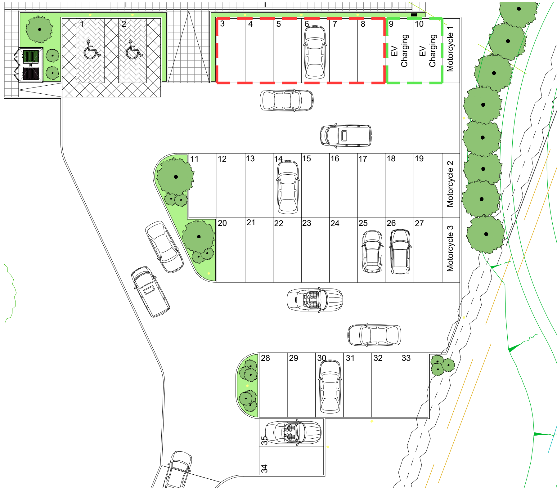
EV Charging Points - Location Plan 1:200
