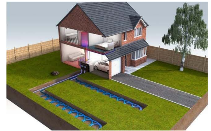
GSHP/Geothermal Floor Panel System
