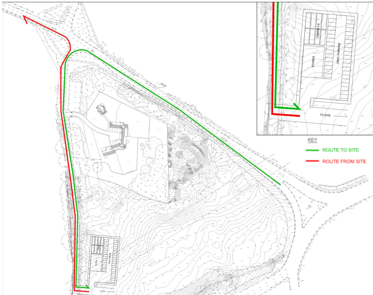
Figure 1.2 – Site Access Route – During Construction
