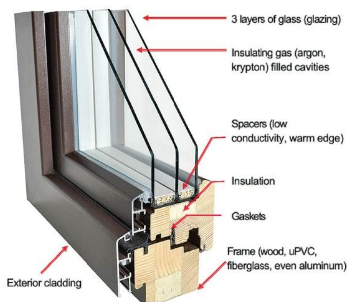
Figure 2. Example Features of a Passive House Window
