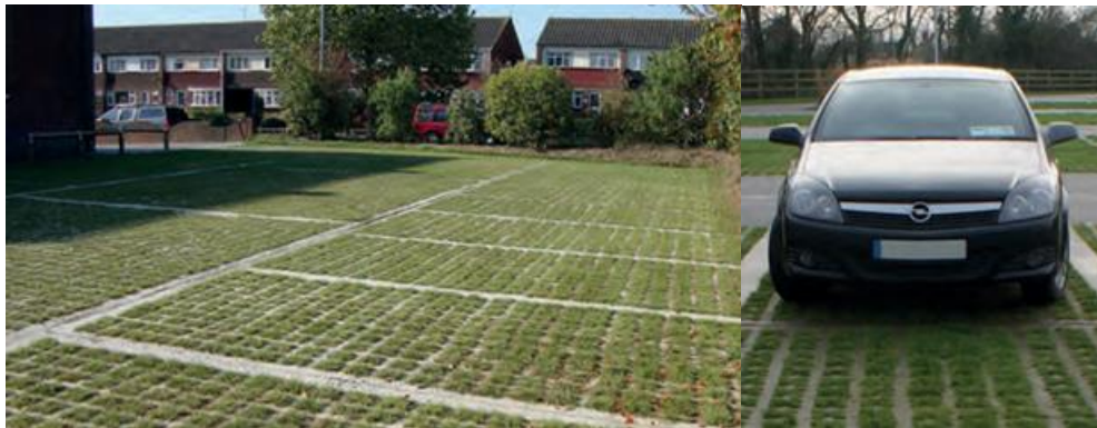
Figure 9 - A Typical Example of Grasscrete parking
