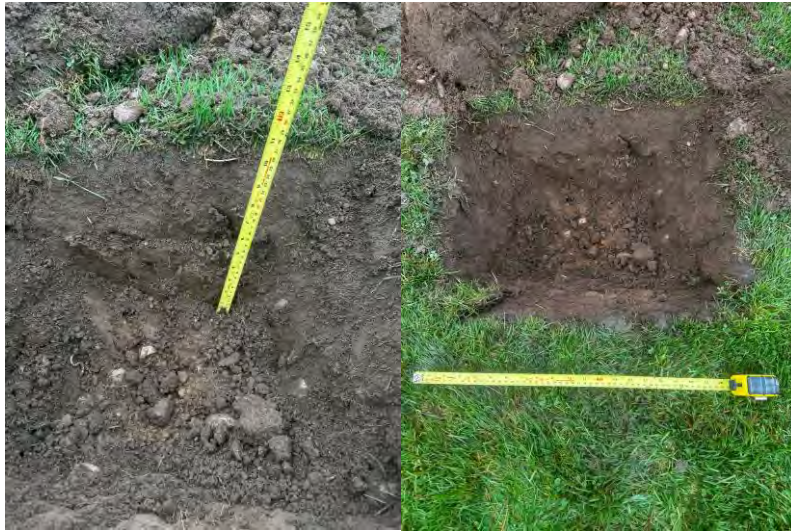
TP7 - 290mm Greyish Brown Sandy Clay Loam Topsoil; Compact; Tree Roots to 150mm; Frequent stones 30-40mm diameter; Worm activity; Dry; Brown Silty Clay Loam Subsoil 290-500mm; No evidence of drainage; End of pit.
