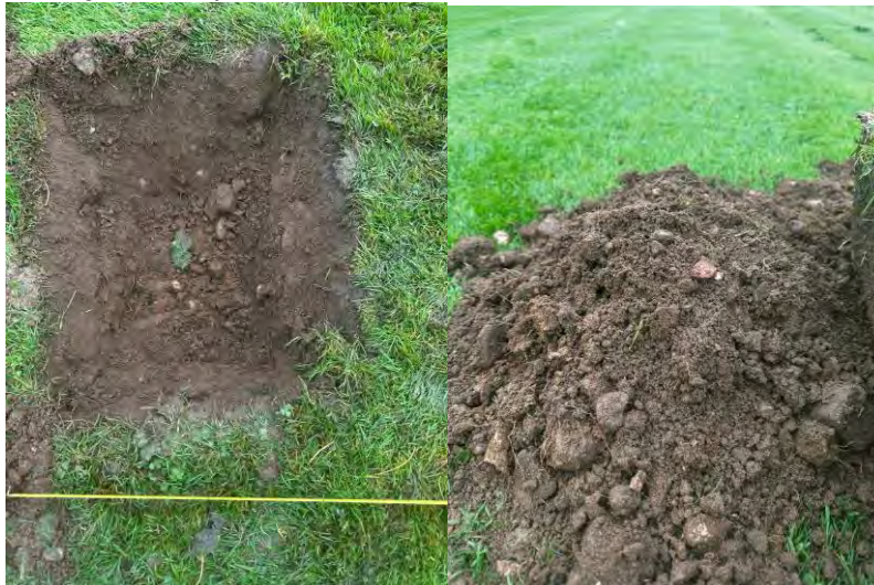
TP8- 290mm Greyish Brown Sandy Clay Loam Topsoil; Compact; Frequent stones 30-40mm diameter; Worm activity; Dry; Brown Silty Clay Loam Subsoil 290-500mm; No evidence of drainage; End of pit.
