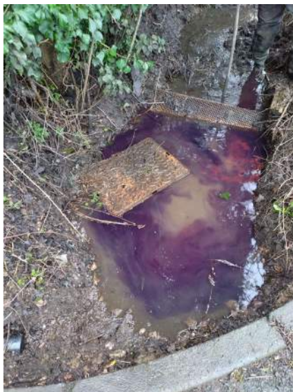
Ditch water dye goes to MH cover edge v.JPG
