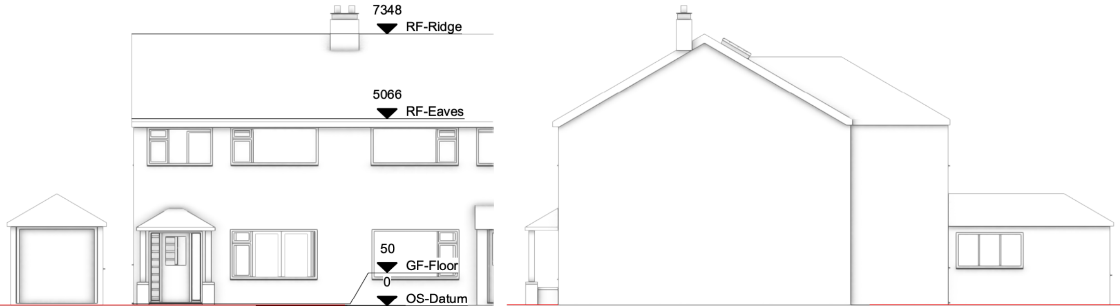
1 North Elevation - Existing Scale: 1:100
