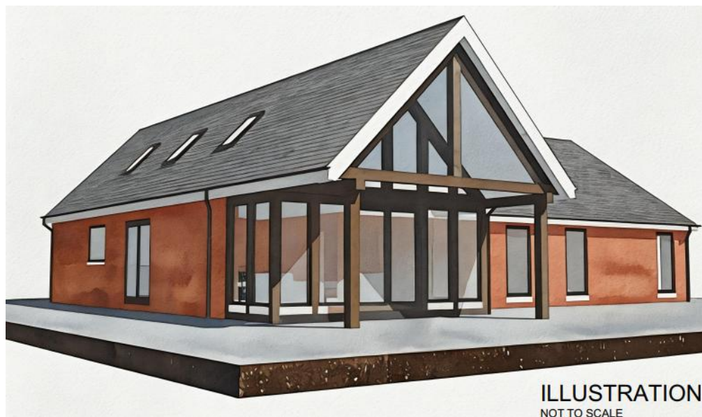
Figure 5 Oak Framed Porch to South Elevation.
