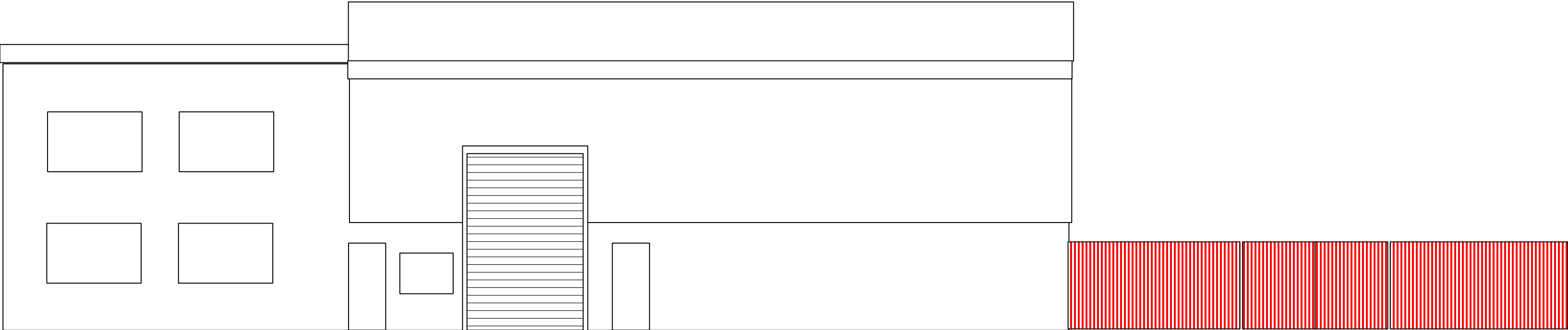
New 2.4 M high Fence and 2.4 High x 4 M Width Gate Mounted at Center of Fence
