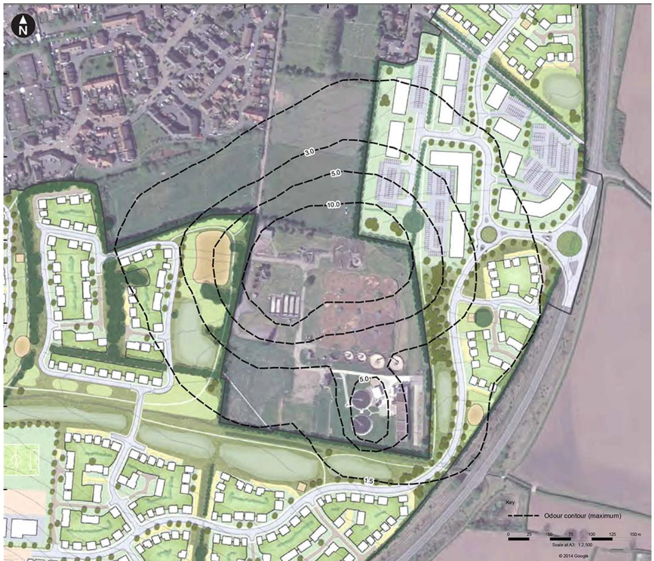
Figure 5-1 - 98 th percentile odour contours ( ou_E/m^3 ) at Earl Shilton STW (maximum over the 2018 to 2022 period)
