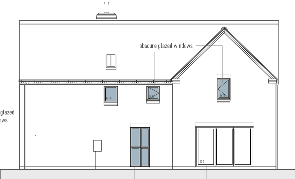
obsure glazed windows door replaced with full height glazed panel Existing bi folds retained side elevation
