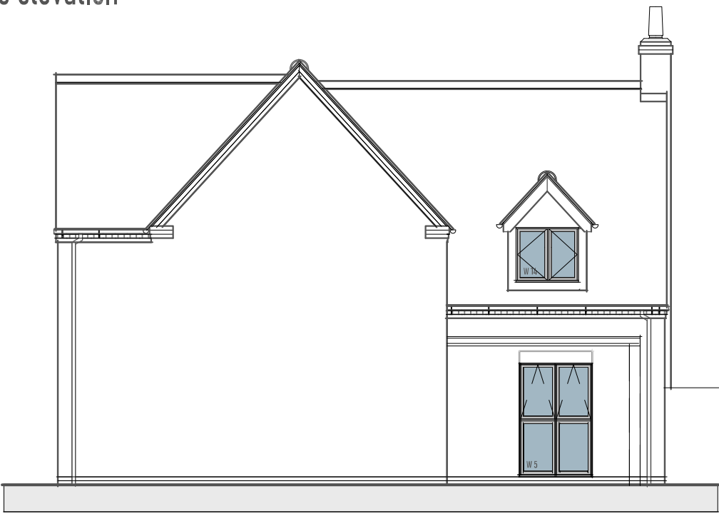
obsure glazed windows door replaced with full height glazed panel Existing bi folds retained side elevation
