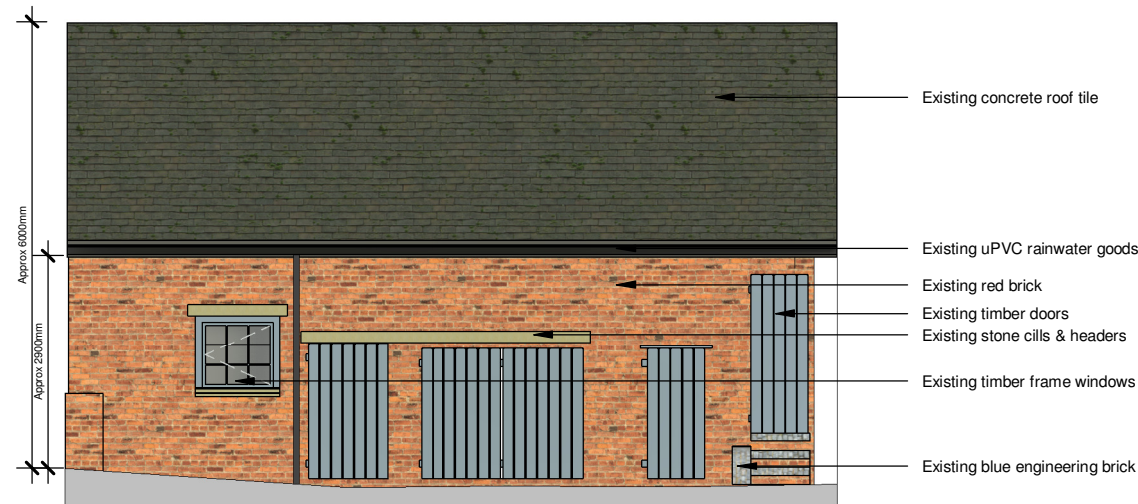
Existing Front Elevation - 1:100
