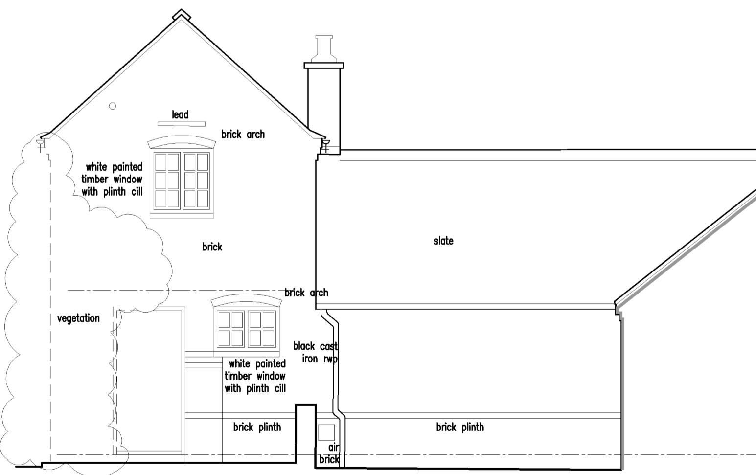
Existing Internal Side Elevation
