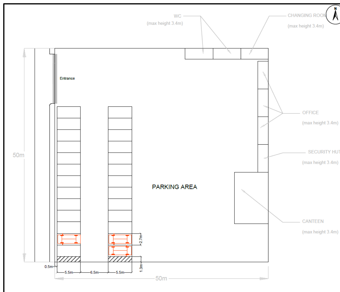
Figure 5: Smaller Temporary Construction Compound
