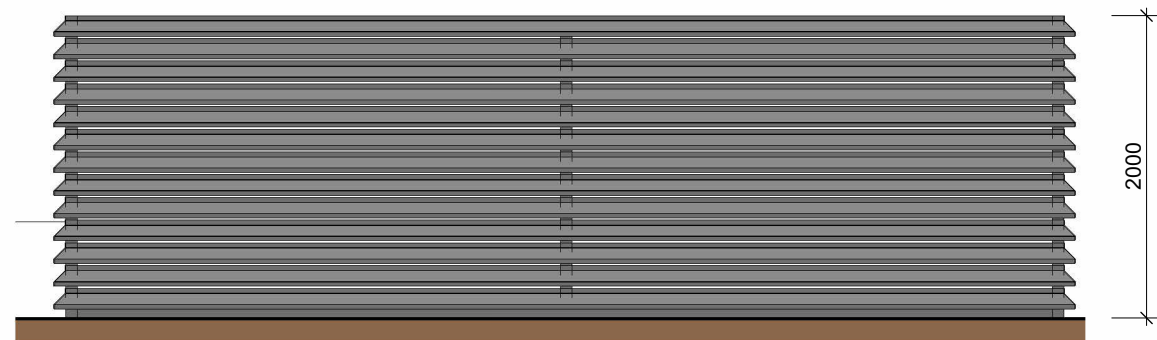
Office Waste Compound - Side Elevation 1 : 50
