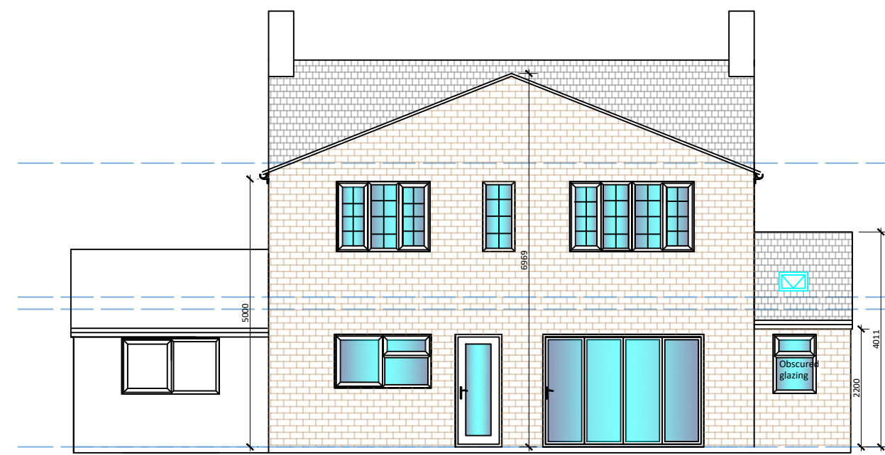
Proposed Rear Elevation @ 1:100
