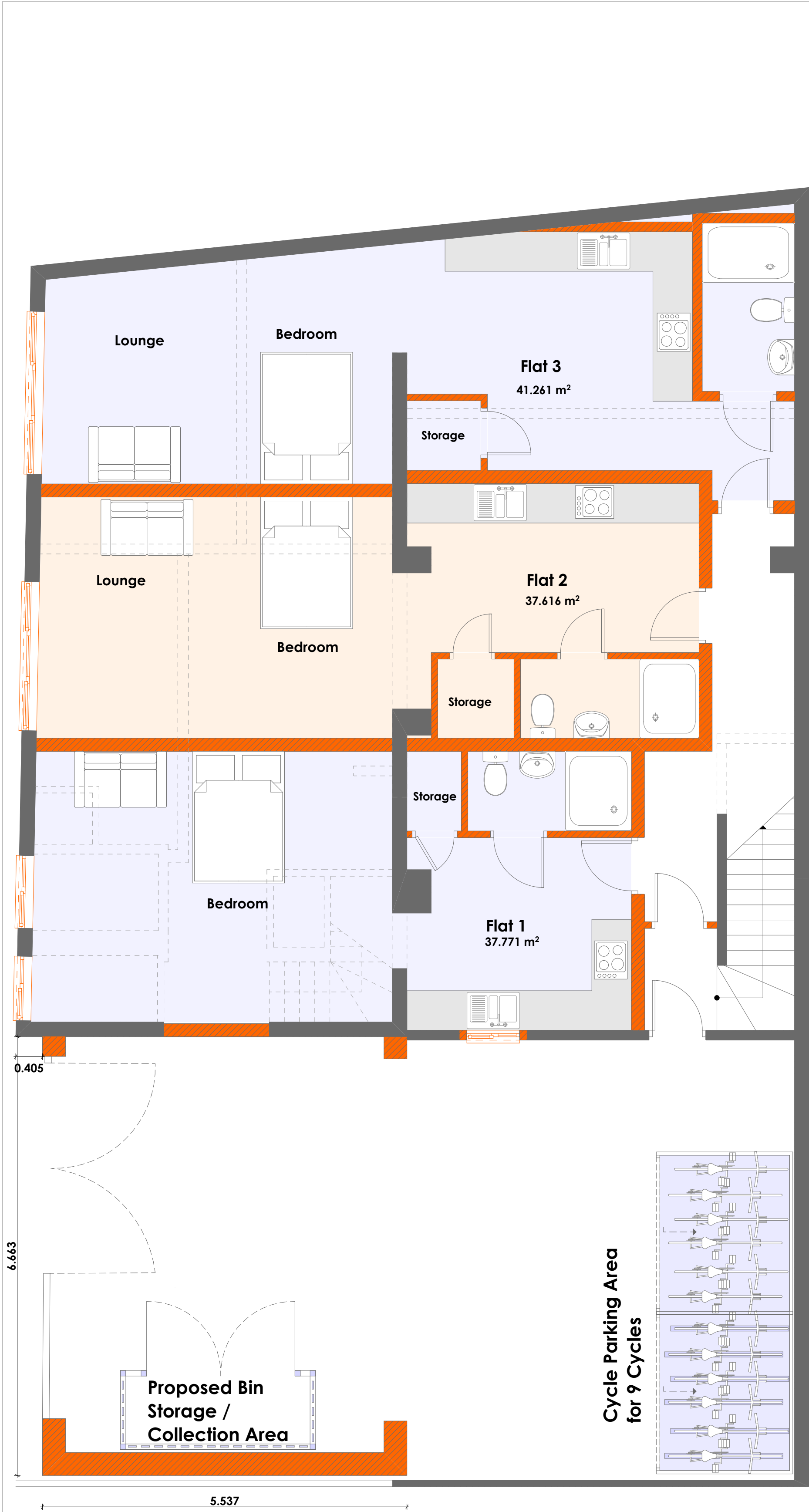
Proposed Ground Floor Plan @1:50
