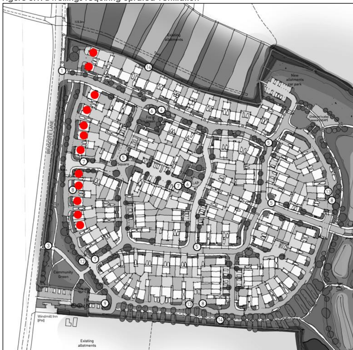
Figure 5.1: Dwellings requiring uprated ventilation
