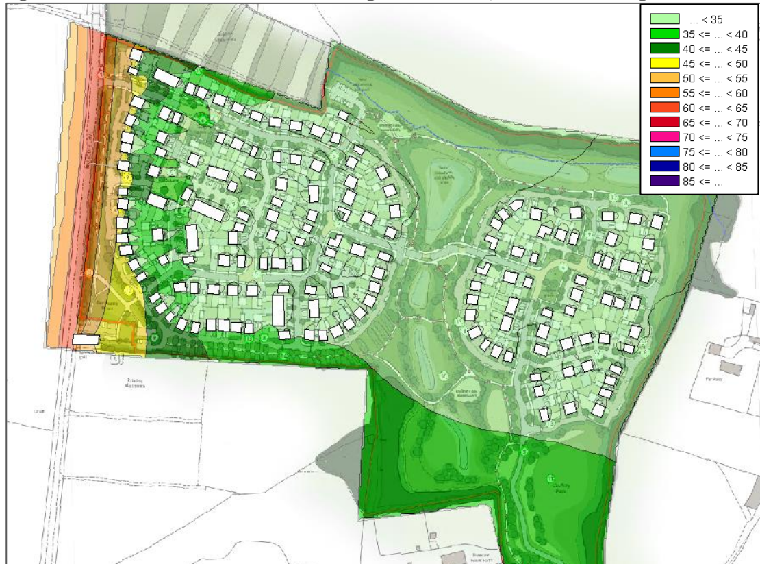
Figure 4.1: Noise Contour Plot without Mitigation, dB L_{Aeq,16h} , 1.5m above ground
