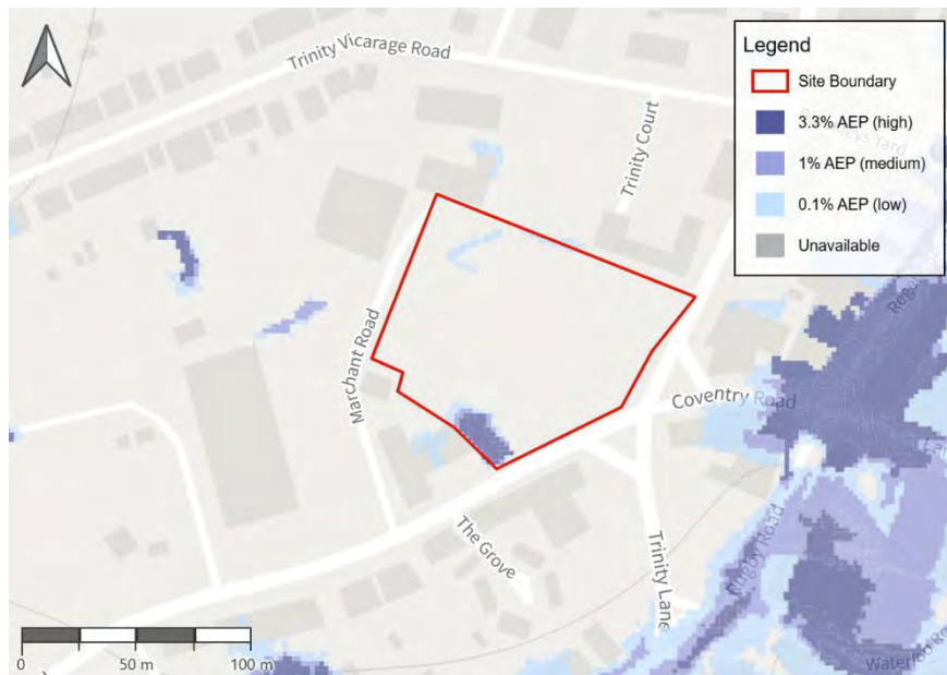
Figure 3 – Pluvial Flooding Extents (EA)
