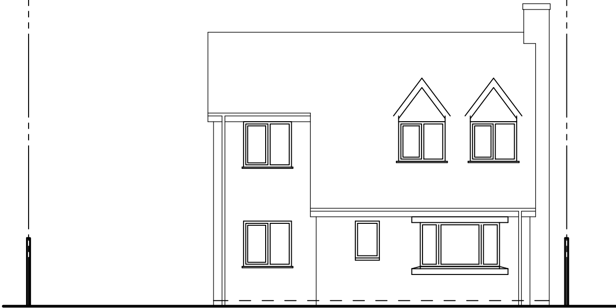
EXISTING FRONT ELEVATION
