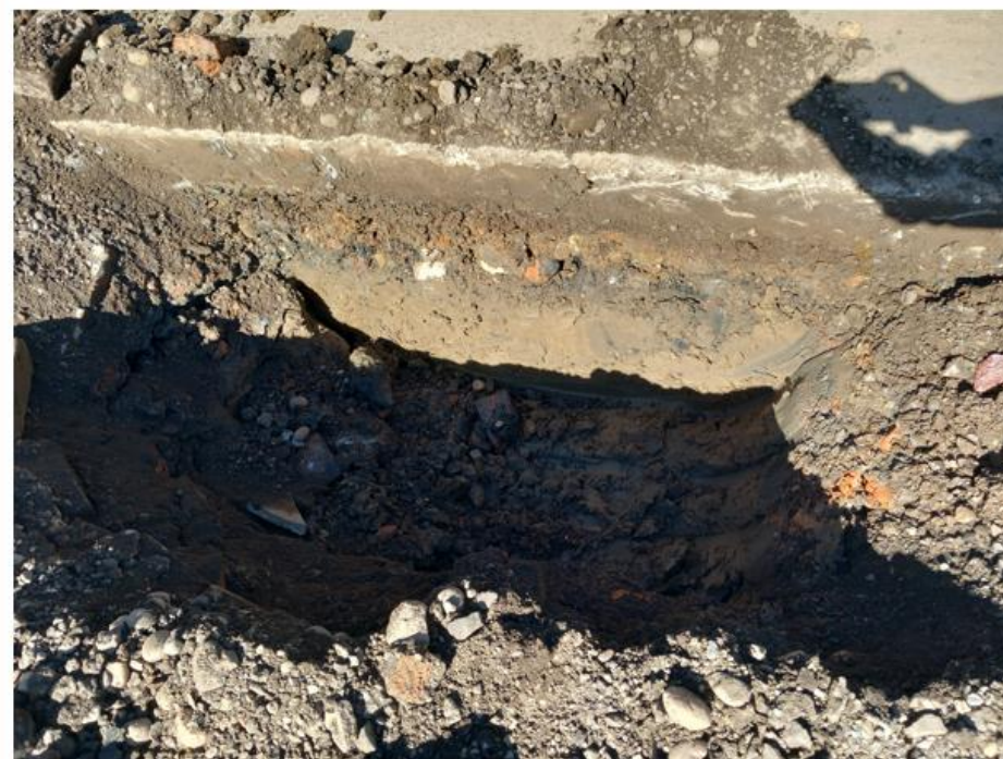
Photo No.4: TP02 pit sides and base (excavated adjacent to existing concrete base) showing made ground atop clays
