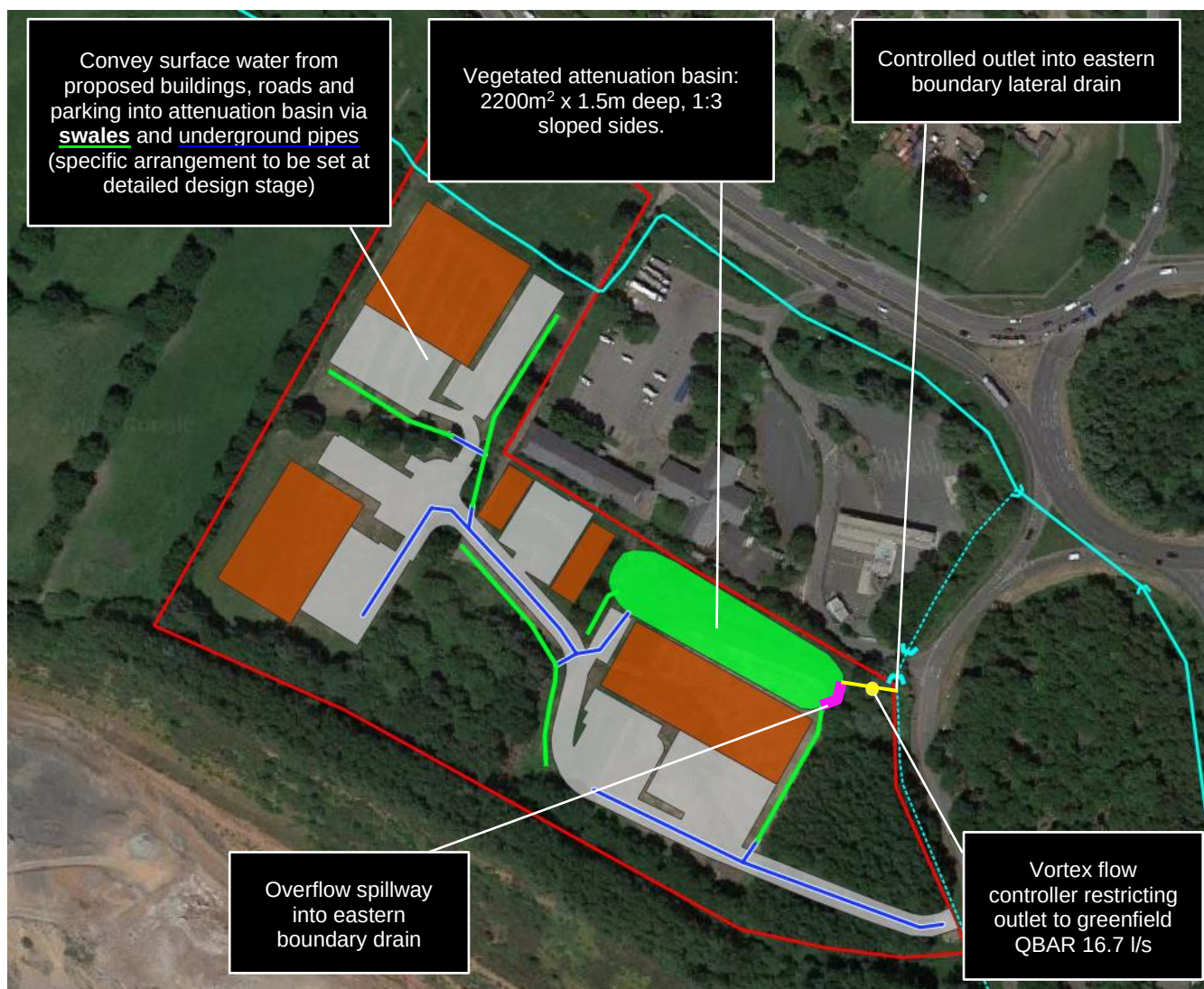
FIGURE 5: PLAN SHOWING THE CONCEPTUAL SURFACE WATER DRAINAGE SCHEME
