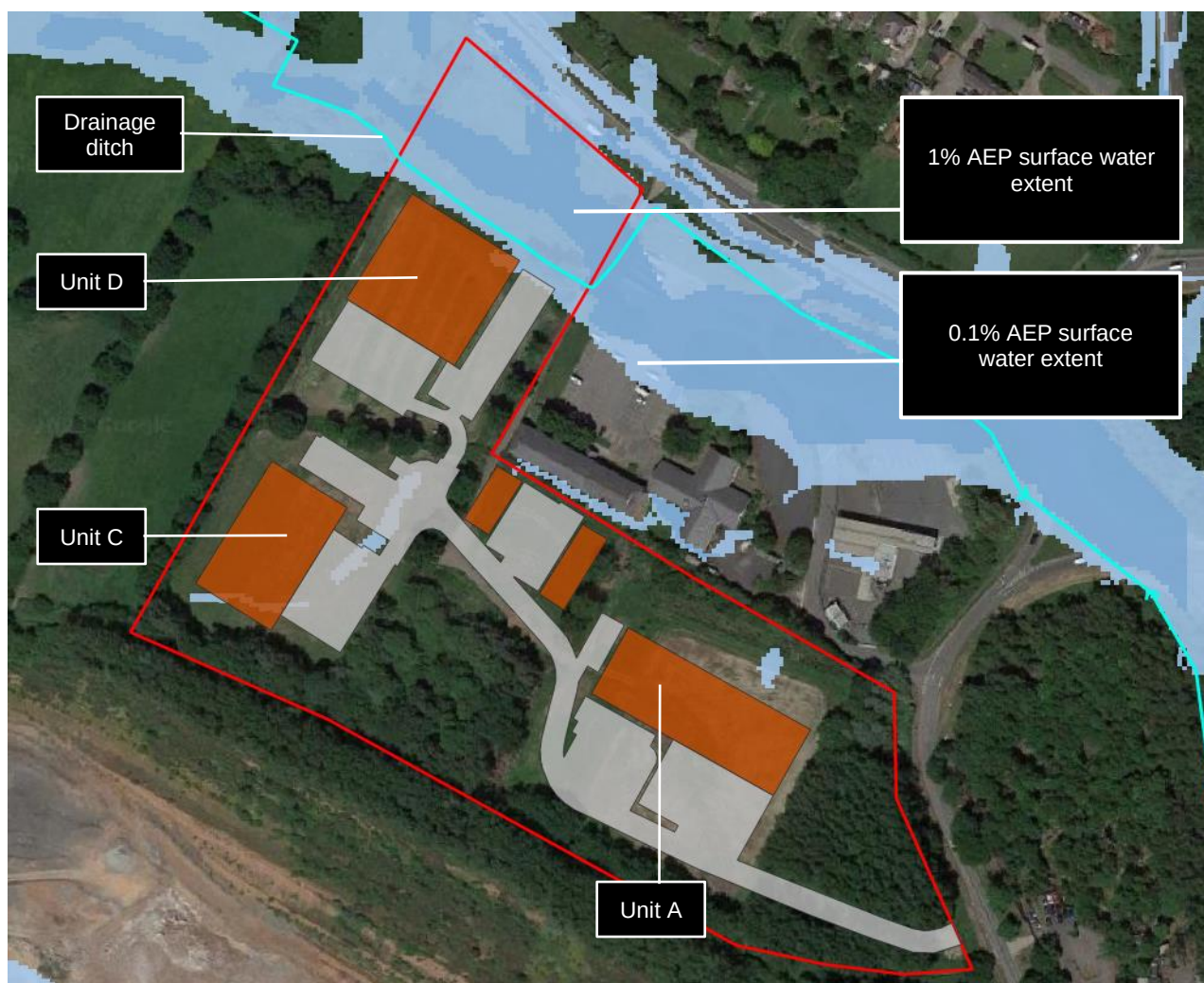
FIGURE 3: SURFACE WATER RISK (1% AEP AND 0.1% AEP EXTENTS) WITH PROPOSED PLAN
