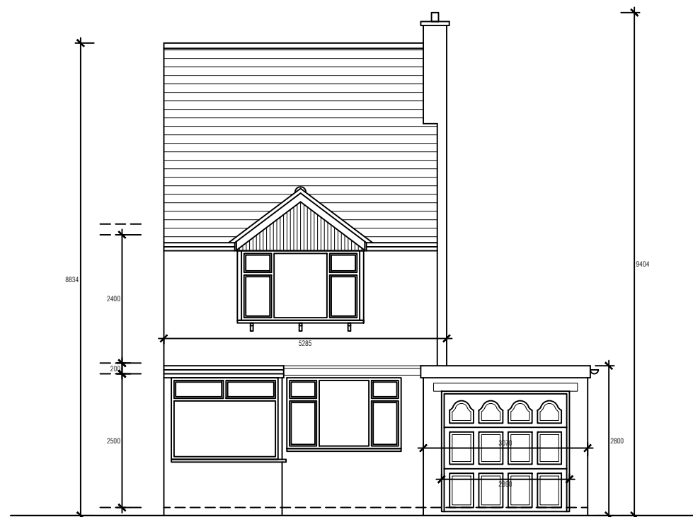
EXISTING FRONT ELEVATION SCALE 1:100
