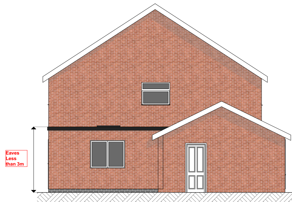
East Elevation - Side
