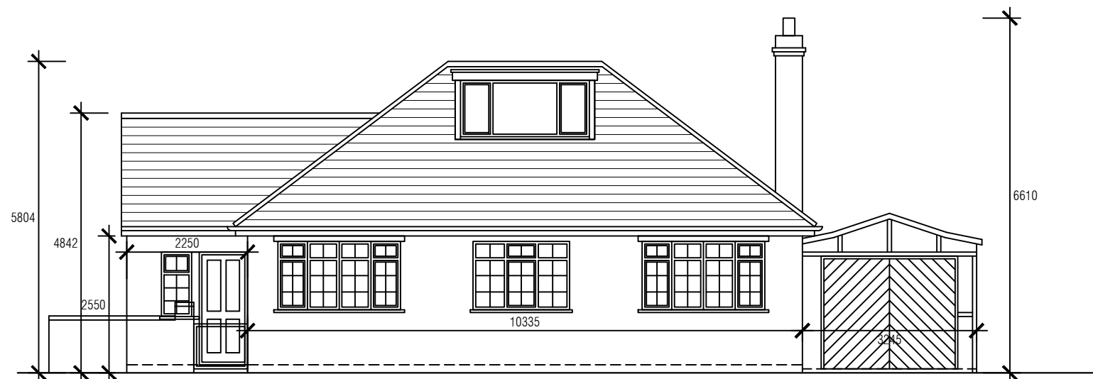
EXISTING FRONT ELEVATION SCALE 1:100
