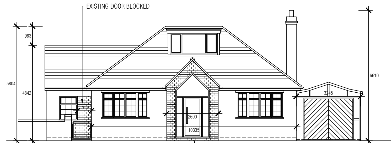
PROPOSED FRONT ELEVATION SCALE 1:100
